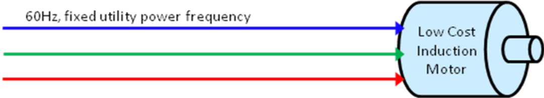
Figure 2. AC Induction Motor Driven by Utility Power Fixed speed, inefficient energy use, quiet operation
